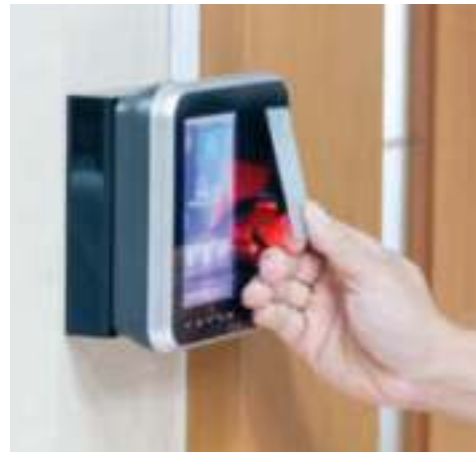
Access Control System
